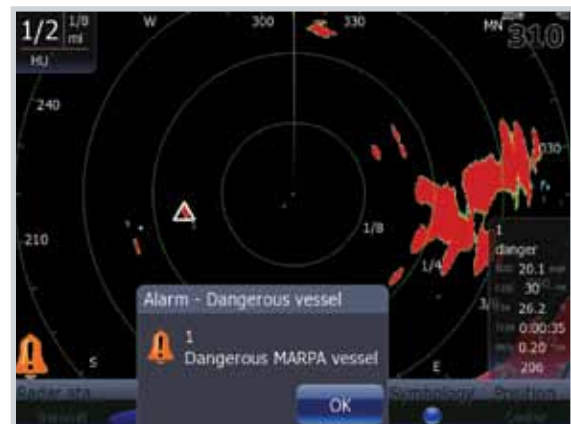
Dangerous vessel incoming at 20.1 mph with 35 seconds to Time to Closest Point of Approach (TCPA).
